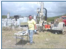
SWMU 78 – Baker Geologist collecting subsurface soil samples
