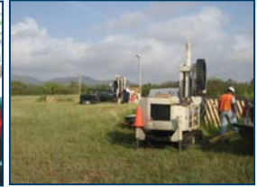
SWMU 74 – Multiple Drill Rigs collecting subsurface soil samples
